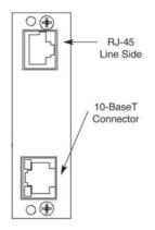
Figure 8. 3088RC/C/AI Ethernet Port
